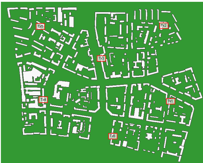
Fig. 1. Model of an urban area used at behavior simulation of cellular system
