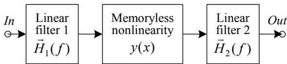
Figure 1. The Wiener–Hammerstein model.
