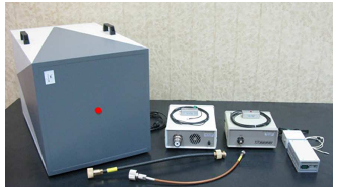
Fig. 1. TS equipment: AFS (left), pulse high-voltage generators (PVGs) 50 kV and 5 kV, high-voltage feeders, DFI (right).
