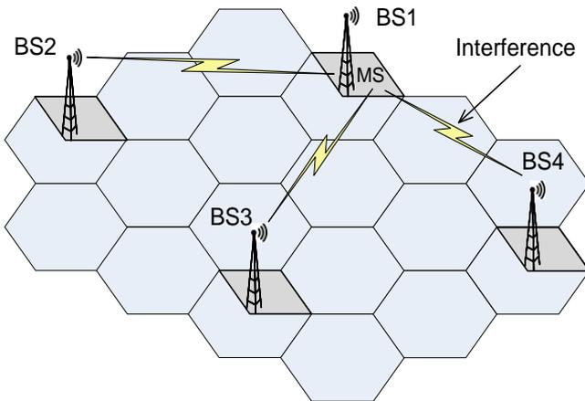
Fig. 1. Scenario of simulation for estimation of CNIR value at the input of MS receivers
