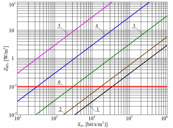
Fig.2. Dependences  $Z_{BS}(S_{tr})$ , obtained for  $R_{max} = 300$  m at different  $K_{CC}$  values and  $Q \approx 1/3$ ,  $S_{EP} = 5$ ,  $K_N = 5$ ,  $T_0 = 290$ K,  $K_H L_m L_C = 50$  dB,  $\lambda = 0.15$  m (2 GHz)
