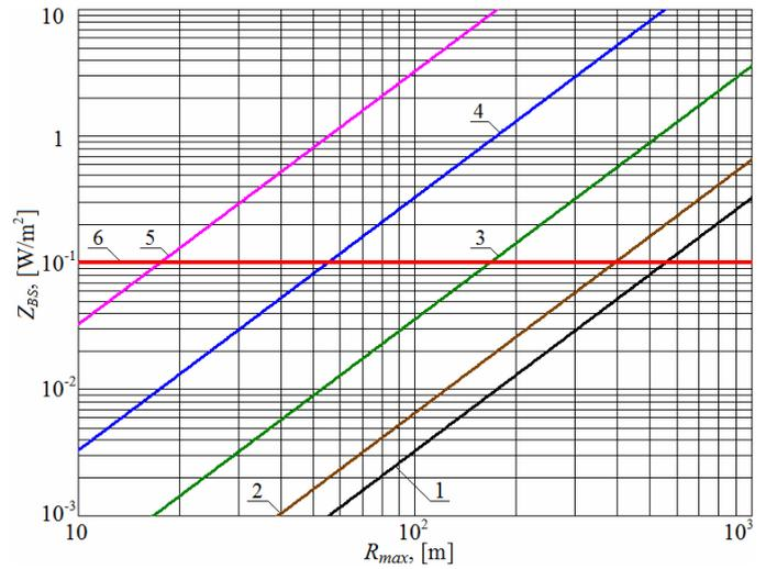
Fig.1. Dependences  $Z_{BS}(R_{max})$  for  $S_{tr} = 10^4$  bit/s/m<sup>2</sup>, obtained for different  $K_{CC}$  values at  $Q \approx 1/3$ ,  $S_{EP} = 5$ ,  $K_N = 5$ ,  $T_0 = 290$ K,  $K_H L_m L_C = 50$  dB,  $\lambda = 0.15$  m (2 GHz)
