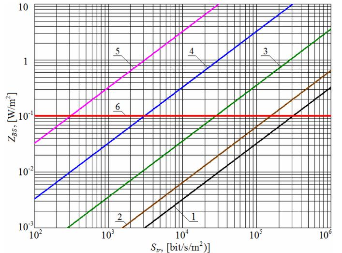
Fig.3. Dependences  $Z_{BS}(S_{tr})$ , obtained for  $R_{max} = 100$  m at different  $K_{CC}$  values and  $Q \approx 1/3$ ,  $S_{EP} = 5$ ,  $K_N = 5$ ,  $T_0 = 290$ K,  $K_H L_m L_C = 50$  dB,  $\lambda = 0.15$  m (2 GHz)
