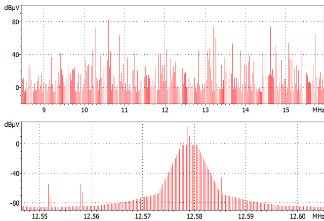
Fig. 6. Spectra of total signal at the input (upper) and output (lower; fed to RR input) of the model of RR belonging to HF radio station; 3rd order intermodulation is observed in the output spectrum close to the adjustment frequency of RR
