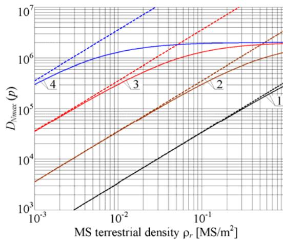
Fig. 2. Dependences of related levels  $D_{Nmax}(p)$  of prevailing EMF of radiating MS nearest to OP, on average terrestrial density  $\rho_r$  of radiating MS, for  $R_{min2} = \lambda/2$  and different  $p$ , considering MS reactive near-field zone (solid lines) and ignoring it (dotted lines)
