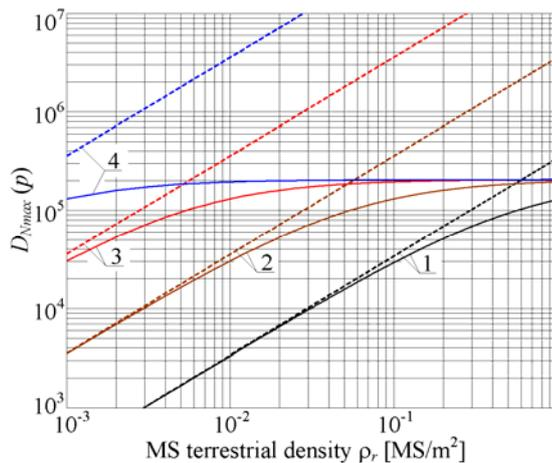
Fig. 3. Dependences of related levels  $D_{Nmax}(p)$  of prevailing EMF of radiating MS nearest to OP, on average terrestrial density  $\rho_r$  of radiating MS, for  $R_{min3} = \pi\lambda/2$  and different  $p$ , considering MS reactive near-field zone (solid lines) and ignoring it (dotted lines)
