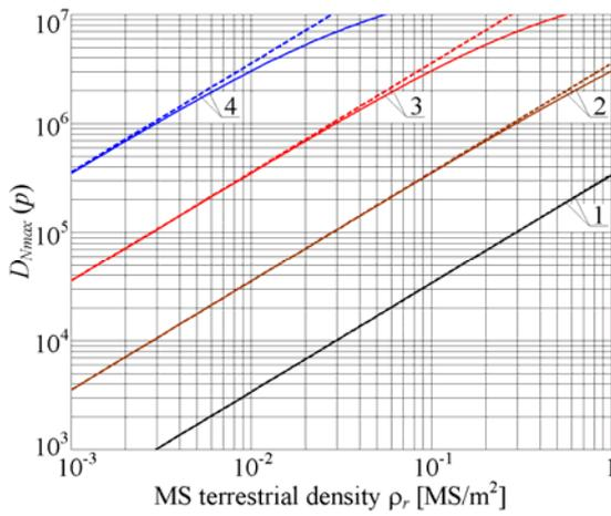
Fig. 1. Dependences of related levels  $D_{Nmax}(p)$  of prevailing EMF of radiating MS nearest to OP, on average terrestrial density  $\rho_r$  of radiating MS, for  $R_{min1} = \lambda/(2\pi)$  and different  $p$ , considering MS reactive near-field zone (solid lines) and ignoring it (dotted lines)
