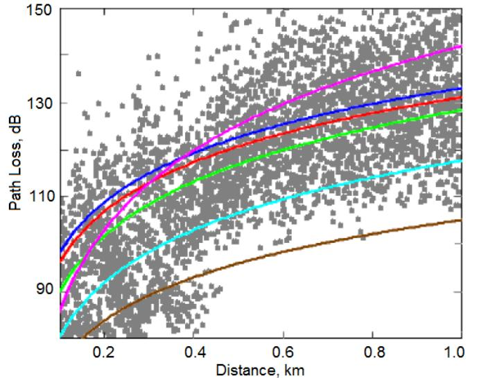
Fig. 3. The example of distribution of values of signal attenuation obtained with usage of 3XD model at BS antenna height  $H_{bs} = 40$  m
