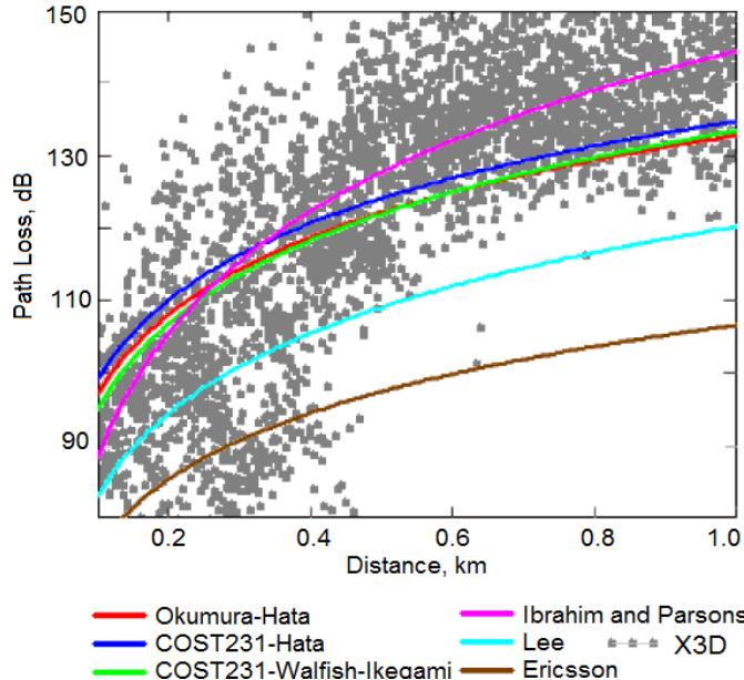
Fig. 2. The example of distribution of values of signal attenuation obtained with usage of 3XD model at BS antenna height  $H_{bs} = 30$  m
