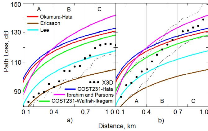
Fig. 6. Dependence of values of signal attenuation from distance between BS and MS at usage of empirical models of RWP and the model of X3D at BS antenna height  $H_{bs} = 40$  m
