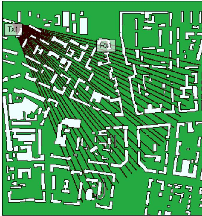
Fig. 1. Model of a fragment of city housing of a central part of Minsk with one BS (Tx1) and MS (Rx1-RxN)
