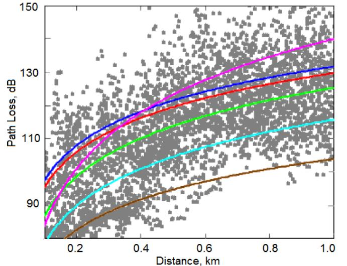
Fig. 4. The example of distribution of values of signal attenuation obtained with usage of 3XD model at BS antenna height  $H_{bs} = 50$  m
