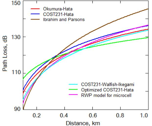
Fig. 8. Dependence of signal attenuation from distance between BS and MS at usage of empirical models and models of RWP for microcell at BS antenna height  $H_{BS} = 30$  m
