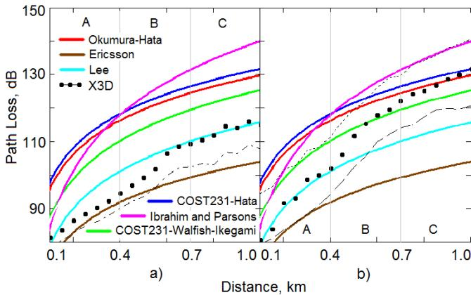
Fig. 7. Dependence of values of signal attenuation from distance between BS and MS at usage of empirical models of RWP and the model of X3D at BS antenna height  $H_{bs} = 50$  m
