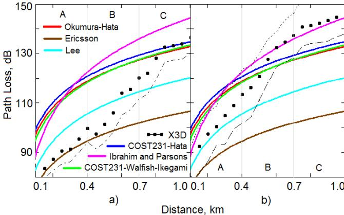
Fig. 5. Dependence of values of signal attenuation from distance between BS and MS at usage of empirical models of RWP and the model of X3D at BS antenna height  $H_{bs} = 30$  m
