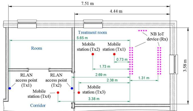
Fig. 3. The allocation of mobile stations and RLAN access points as emitters and NB IoT devices as receptors
