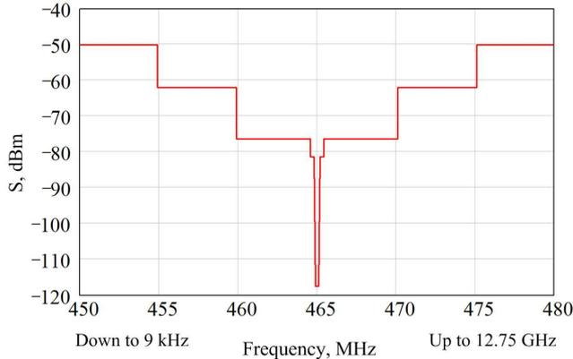
Fig. 2. Susceptibility mask of NB IoT user equipment receiver
