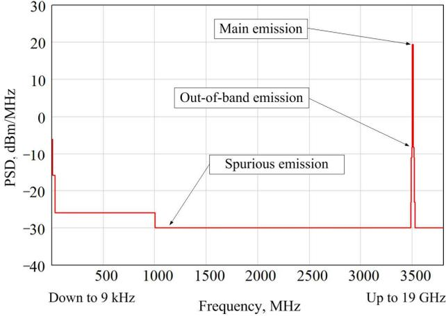
Fig. 1. Spectrum mask of 5G mobile station transmitter
