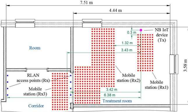
Fig. 4. The allocation of NB IoT device as emitter and mobile stations and RLAN access points as receptors
