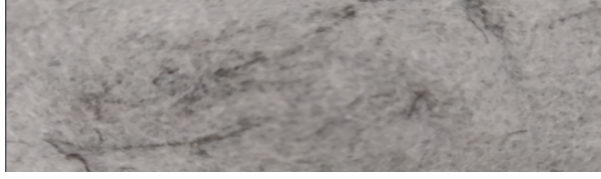
Fig. 7. Structure of a needle-punched material containing carbon fibers
