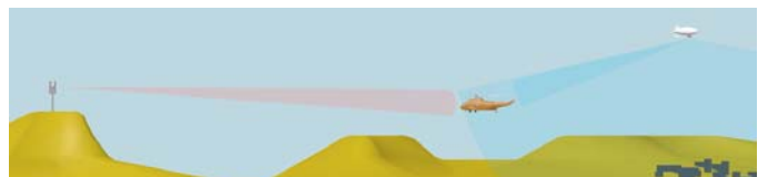
Fig. 2. Layout of interference emitters and receptor.
